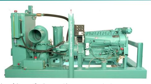
our wellpoint pumps is independent of the centrifugal pump, with no cross contamination to wear on vacuum pump tolerances.
